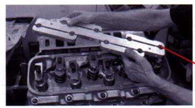
Now with stud girdle loosely fastened together, place it 1st on the intake poly lock and use this poly lock as a pivot point.
