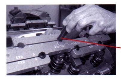
Next simply slide the intake poly locks through the girdle and rough adjust the vave lash.
